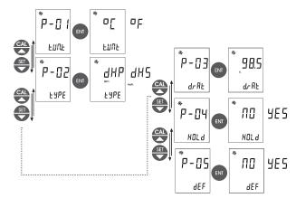
P01: Unit of the temperature. You can select between  $^{\circ}\text{C}$  and  $^{\circ}\text{F}.$
